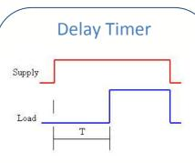
Upon application of power the timer resets, enters the OFF state for a period T, then switches ON indefinitely.
